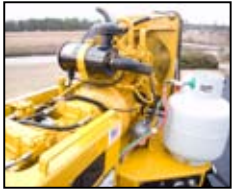
The 38 HP diesel engine provides ample power for paving steep paths.
